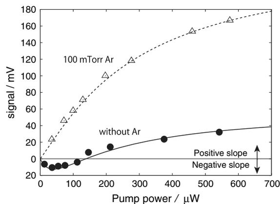
Fig. 3. Dependence of the dispersion signal at the cooling transition on the pump power. The vertical axis represents the peak-to-peak amplitude of the dispersion signal. The open triangles and the solid circles represent the experimental data at zero and 100 mTorr Ar buffer gas pressures, respectively. The solid curve and the dashed curve show calculations for each condition.
