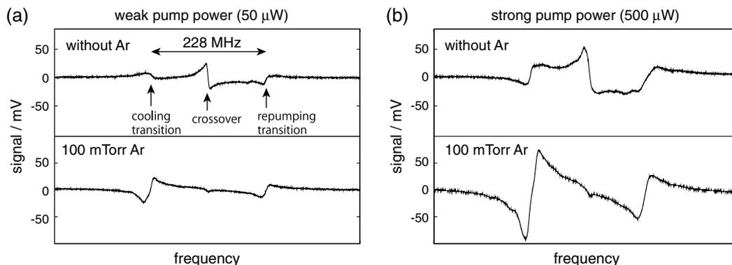
Fig. 2. Doppler-free polarization spectra of the  $2S_{1/2} \rightarrow 2P_{3/2}$  transitions of  ${}^6\text{Li}$  at zero and 100 mTorr Ar buffer gas pressures for (a) a weak ( $50 \mu\text{W}$ ) and (b) a strong ( $500 \mu\text{W}$ ) pump power.
