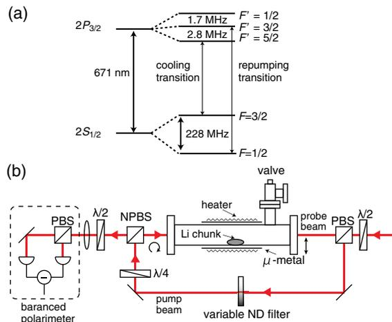
Fig. 1. (Color online) (a) Relevant  ${}^6\text{Li}$  energy levels. (b) Schematic diagram of the experimental setup. PBS, polarization beam splitter; NPBS, nonpolarization beam splitter;  $\lambda/2$ , half-wave plate;  $\lambda/4$ , quarter-wave plate; ND filter, neutral density filter.
