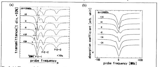
Fig. 2. (a) The transmission spectra around F=2-F'=1 transition for various repumping laser detunings. (b) Calculated spectra corresponding to the experimental results by using the density-matrix formalism of a two-level system.
