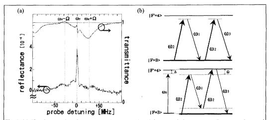
Fig. 3. (a) The phase-conjugation spectrum (upper trace) and the transmission spectrum (lower trace) around the trapping laser frequency. (b) The schemes for degenerate (upper part) and nearly-degenerate (lower part) four-wave mixing.
