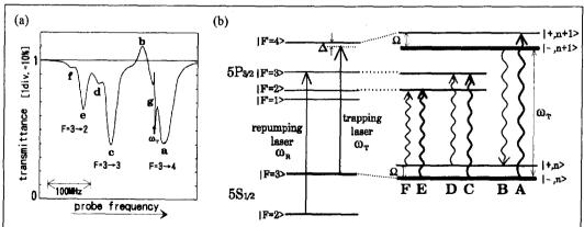
Fig. 1. (a)The transmission spectrum around F=3-F'=2,3,4 transitions. (b) Explanation of the spectral features with a dressed-atom picture.  $\Omega$  is the generalized Rabi frequency defined as  $\Omega^2 = \Delta^2 + \Omega_0^2$ , where  $\Delta$  is the detuning of the trapping laser  $\omega_T$  from the F=3-F'=4 transition and  $\Omega_0$  is resonant Rabi frequency of trapping laser. The lines representing energy levels have widths indicating their relative population.
