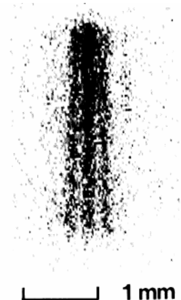
FIG. 2. The interference fringe pattern on the MCP for atoms with the initial velocity of approximately zero. The vertical length of the slit image is 2.8 mm. The spatial resolution of the picture is 20 and 32 \mu\text{m} for the horizontal and vertical directions, respectively. The narrowing of the fringe separation on the upper part is due to the damage of the double-slit structure. This figure contains approximately 6 \times 10^3 atomic counts.
