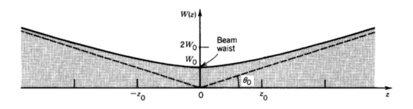
$$w(z) \equiv w_0 \left[ 1 + \left( \frac{z}{z_0} \right)^2 \right]^{1/2} \quad w_0 = \left( \frac{\lambda z_0}{\pi} \right)^{1/2} \text{ ibeam waist}$$
