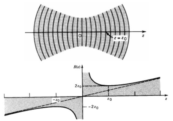
$$R(z) \equiv z \left[ 1 + \left( \frac{z_0}{z} \right)^2 \right] \xrightarrow{z >> z_0} z \qquad u \propto \exp \left[ ik \left( z + \frac{\rho^2}{2z} \right) \right]$$
