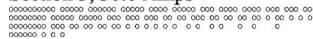
FIG. 11. Winding pattern cross section for the 87 Rb Zeeman slower consisting of three solenoids. Each drawing represents half of the cross section of each a solenoid. The “O”s represent wires, while the spaces between the wires were meant to be smoothed out to an average value during construction. Each character in the drawing represents a physical size of 3.5 mm. The wire is hollow core water-cooled copper, identical to that used in construction of the magnetic trap as described in Appendix C 3. The high current coil is closest to the main chamber. The single layer uniform bias coil is not depicted.
